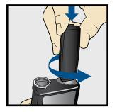
1. Unscrew the battery cap using the bottom edge of the belt clip. (Or use a thick coin.)
