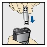
2. Insert battery with negative (flat) end going in first.
